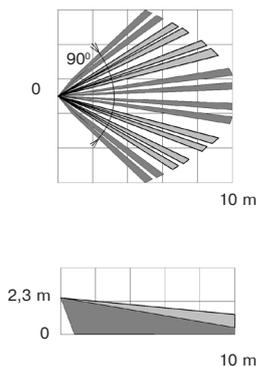
Figure 1 – PIR channel detection zone pattern
