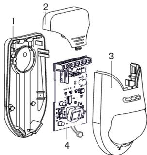
Figure 3 – The Detector Design
