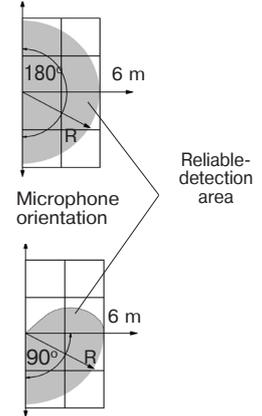
Figure 2 – GB channel detection zone pattern
