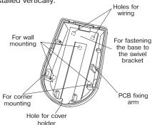
Figure 2 - Base of the Detector
