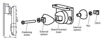
Figure 4 - Swivel bracket fastening and mounting
