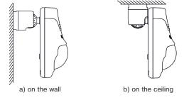
Figure 4 - The Detector mounted on swivel bracket
