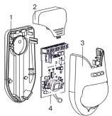
Figure 3 - The Detector Design
