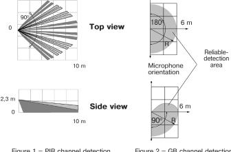
Figure 1 - PIR channel detection zone pattern
